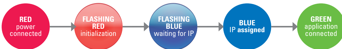
Device status indicated by external LED
